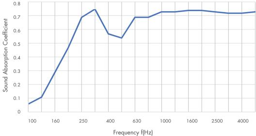
The graph above presents third octave sound absorption coefficients in accordance with ISO 354 measurement of sound absorption in a reverberation room. The table below presents the practical sound absorption coefficients in accordance with ISO 11654. The NRC rating is determined as the arithmetic average of the absorption coefficients measured by one-third octave bands centered on 250 Hz, 500 Hz, 1000 Hz and 2000 Hz and rounded to the nearest 0.05.
