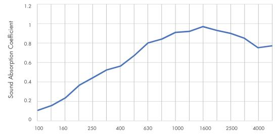
The graph above presents third octave sound absorption coefficients in accordance with ISO 354 measurement of sound absorption in a reverberation room. The table below presents the practical sound absorption coefficients in accordance with ISO 11654. The NRC rating is determined as the arithmetic average of the absorption coefficients measured by one-third octave bands centered on 250 Hz, 500 Hz, 1000 Hz and 2000 Hz and rounded to the nearest 0.05.
